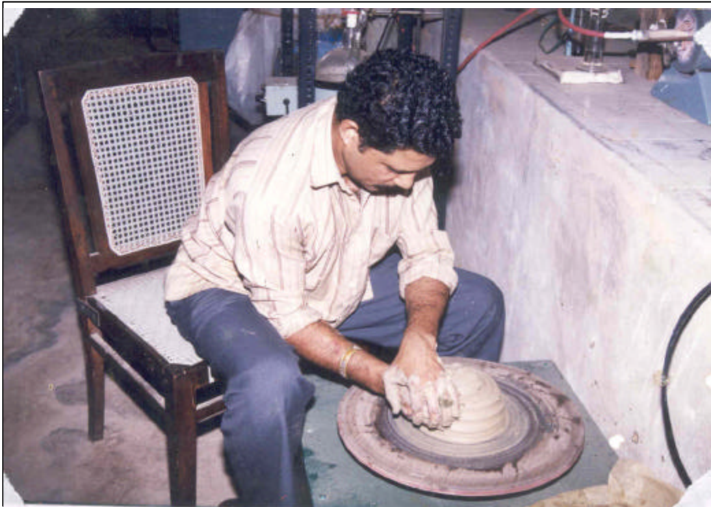
Fig. 4.4. Pottery expert Sri. Susheel checking the performance of the motorised potters' wheel
