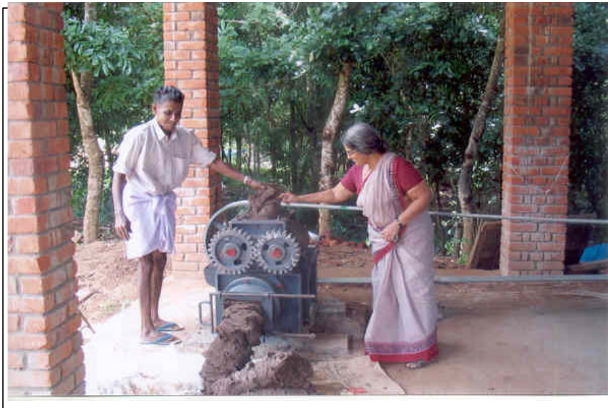
Fig. 4.9. Shri. G. Baby Preparing pugged clay to be used on the potters' wheel
